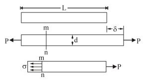
A section taken perpendicular to longitudinal axis of bar is cross-section. Considering free-body diagram, the tensile force P acts on right hand of free body at the other end is force representing the action of removed part of bar upon the part that remains. These forces are continuously distributed over the cross-section. The intensity of force (i.e. force per unit area) is called the stress and is denoted by
