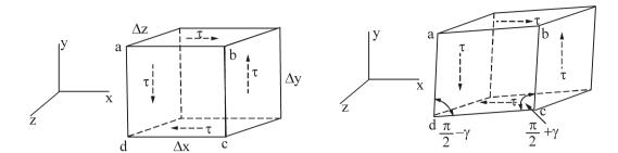
Considering force equilibrium, total shear force on the top face is  $\tau\Delta x\Delta z$  and this force is balanced by equal and opposite force on bottom face. These two forces form a couple having moment about z-axis of magnitude  $\tau\Delta x\Delta y\Delta z$ . Equilibrium of element requires this moment to be balanced by equal and opposite moment resulting from shear stress acting on side face of element.
