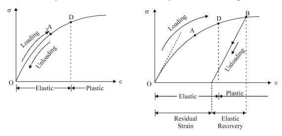
Suppose material is loaded and strain go from O to A. When load is removed, the material follows exactly the same curve back to origin O. This Property of material by which it returns to its original dimension during unloading is called elasticity and material is said to be elastic.
